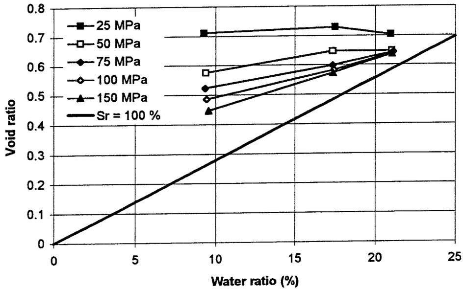
Figure 4-10. The void ratio as a function of water ratio for MX-80 after removal from the form. Compaction pressure 25 - 150 MPa.
