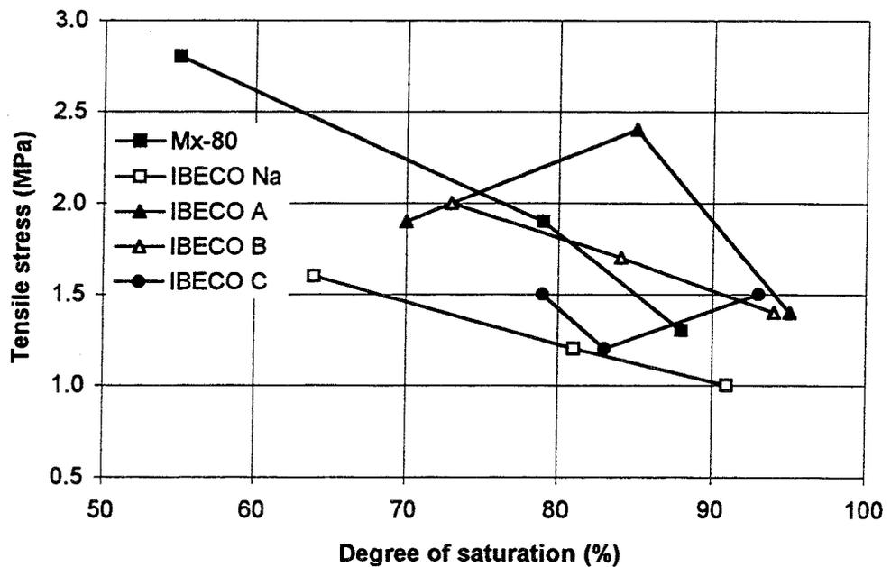
Figure 6-6. Tensile stress at failure as a function of degree of saturation for different bentonites.
