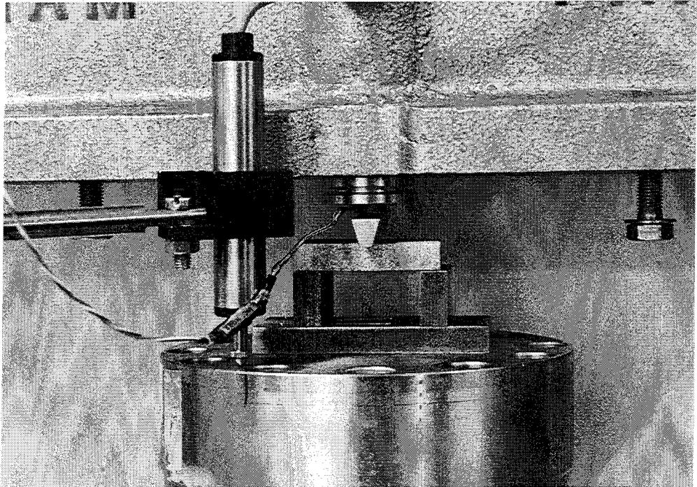
*Figure 6-3. Test arrangement for determination of the tensile strength.*
