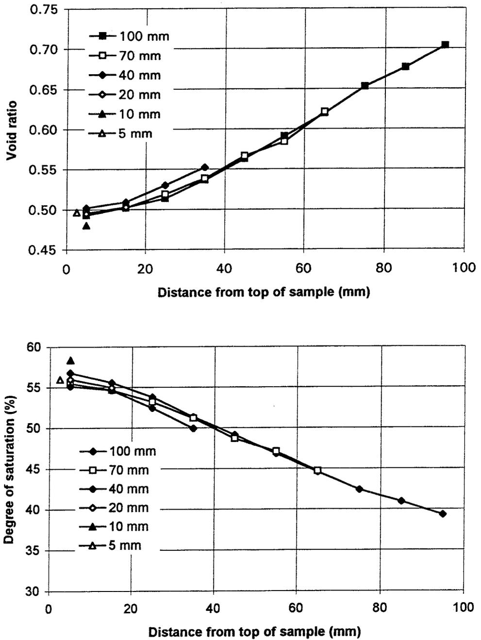
*Figure 4-4. Void ratio (a) and degree of saturation (b), plotted as functions of the distance from the top surface of the sample for different sample heights. Water ratio = 10%.*
