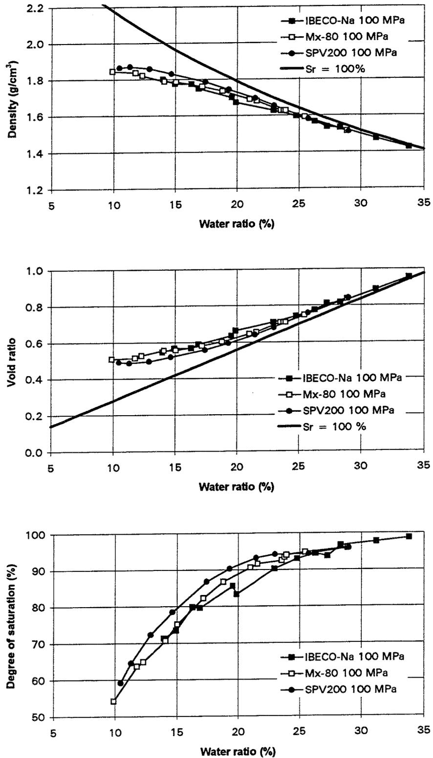
*Figure 4-2. Dry density (a), void ratio (b), and degree of saturation (c) plotted as functions of water ratio for three bentonites. Compaction pressure = 100 MPa.*
