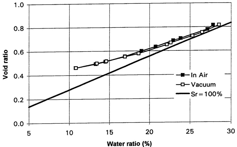
*Figure 4-16. Void ratio as a function of water ratio for samples compacted in air and during vacuum.*
