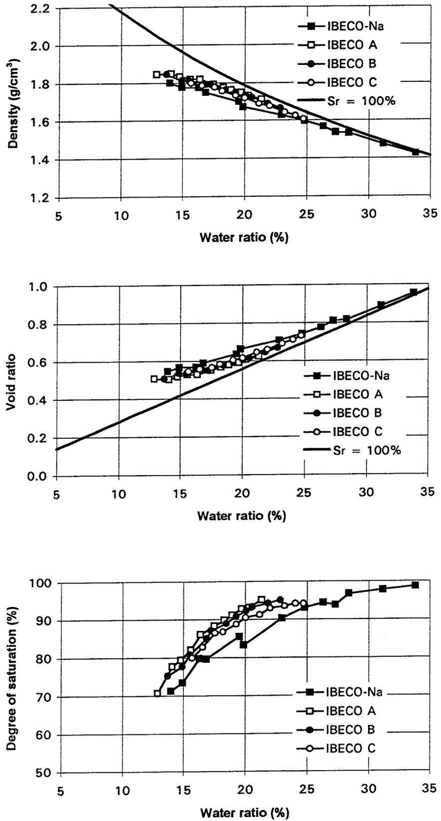
Figure 4-3. Dry density (a), void ratio (b), and degree of saturation (c) plotted as functions of water ratio for four types of IBECO bentonite. Compaction pressure = 100 MPa.
