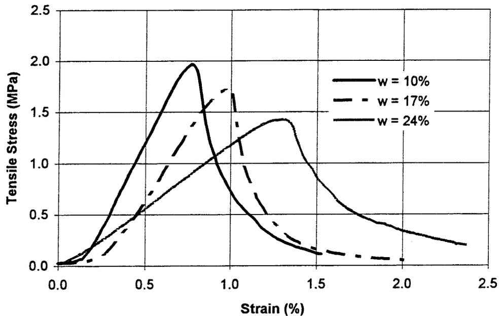
*Figure 6-4. Example of stress/strain relations measured during the tensile strength tests on IBECO B.*
