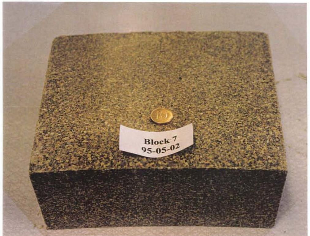
**Figure 7-1. Example of a block compacted at Höganäs Bjuf AB**
