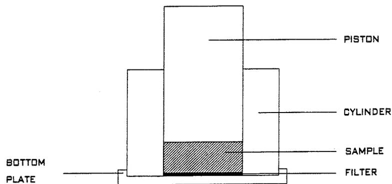
*Figure 3-1. Schematic drawing of the compaction cylinder.*
