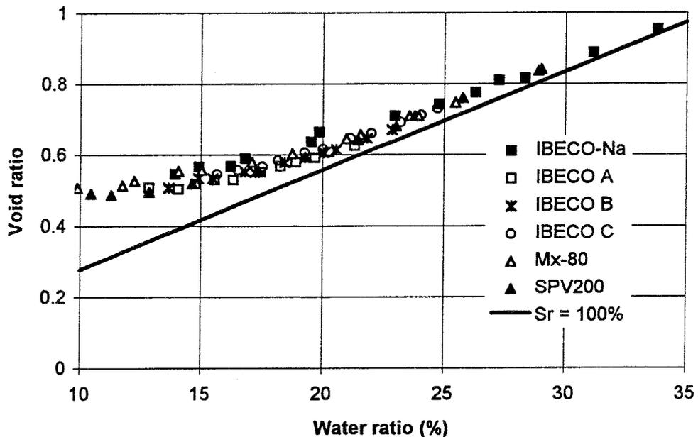
*Figure 4-12. The void ratio as a function of water ratio for different types of bentonites.*
