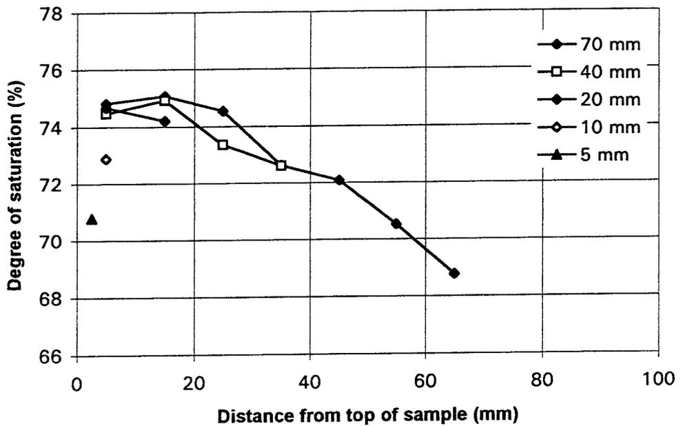
*Figure 4-5. Void ratio (a) and degree of saturation (b), plotted as functions of the distance from the top surface of the sample for different sample heights. Water ratio = 15%.*
