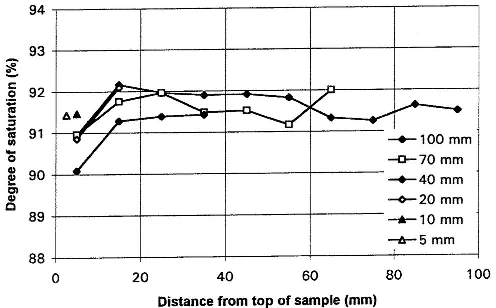
*Figure 4-7. Void ratio (a) and degree of saturation (b), plotted as functions of the distance from the top surface of the sample for different sample heights. Water ratio = 22%.*
