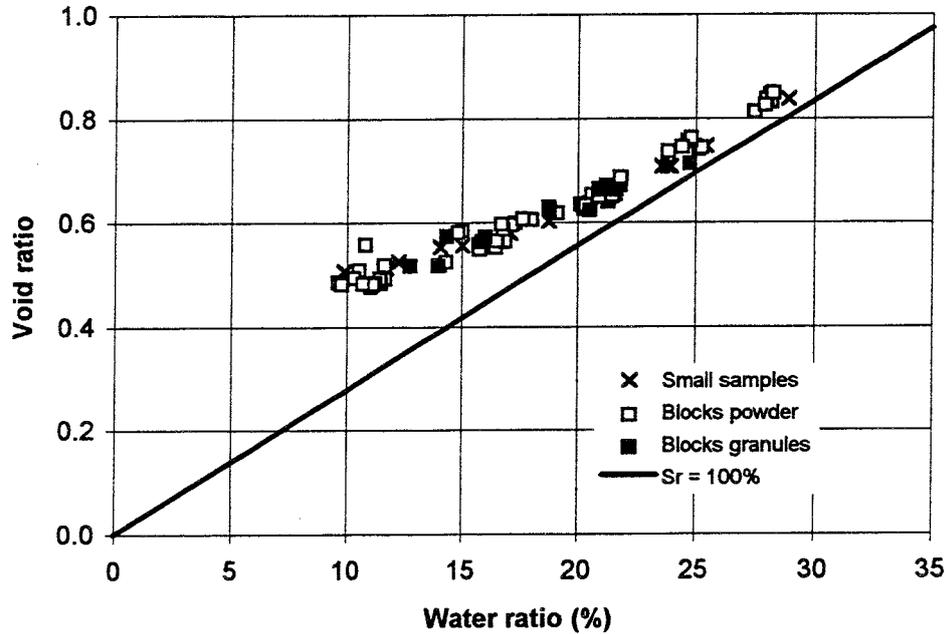
*Figure 6-1. Compilation of compaction results. Void ratio as a function of water ratio for blocks and small samples ( $\Phi = 35$  mm).*
