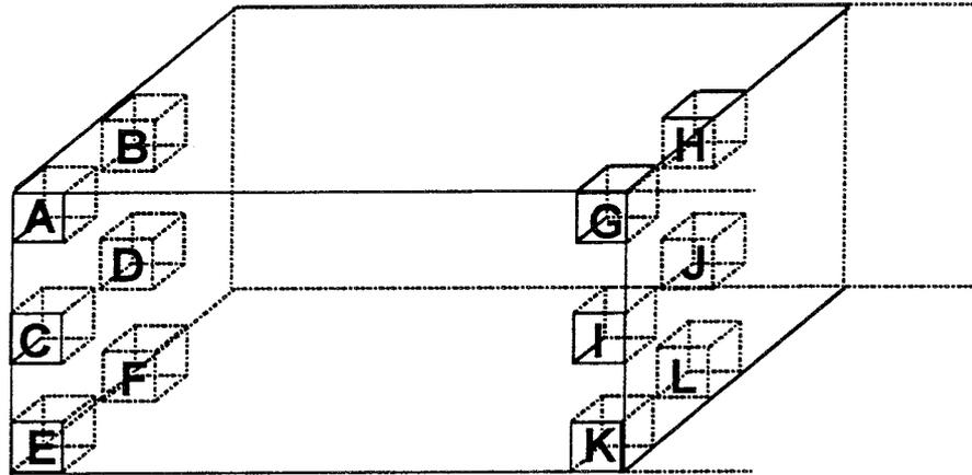
*Figure 6-2. The locations within a block where the density and water ratio were measured. Only half of the block is shown.*
