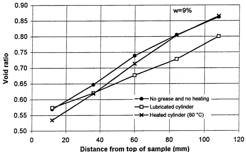
*Figure 4-14. The void ratio as a function of the distance from the top surface of the samples. Water ratio = 9%.*
