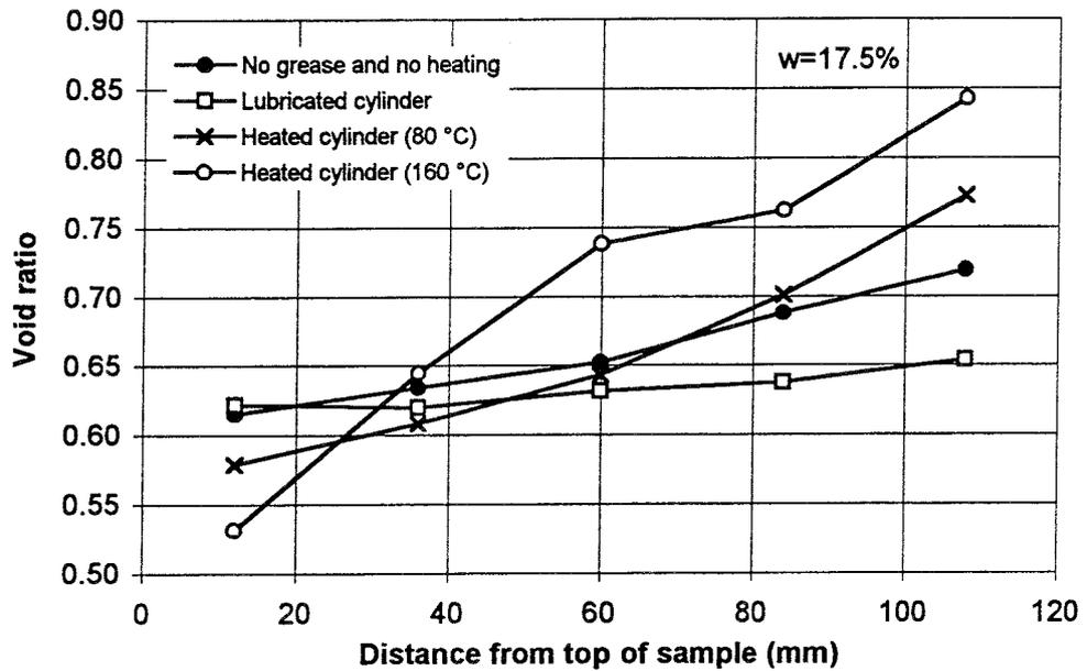
*Figure 4-15. The void ratio as function of the distance from the top surface of the samples. Water ratio = 18%.*
