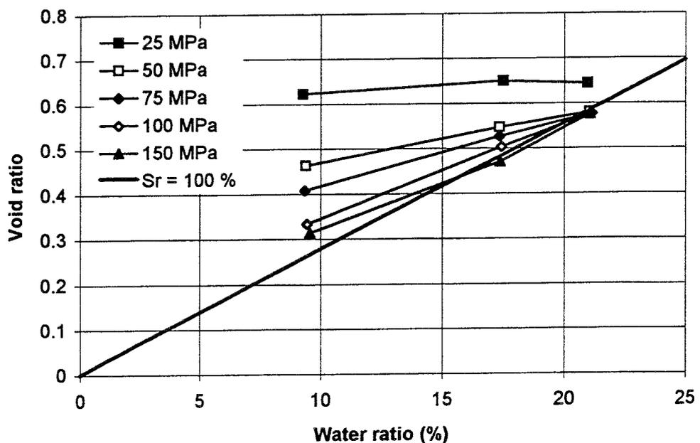
*Figure 4-9. The void ratio as a function of water ratio for MX-80 during compaction. Compaction pressure 25 - 150 MPa.*
