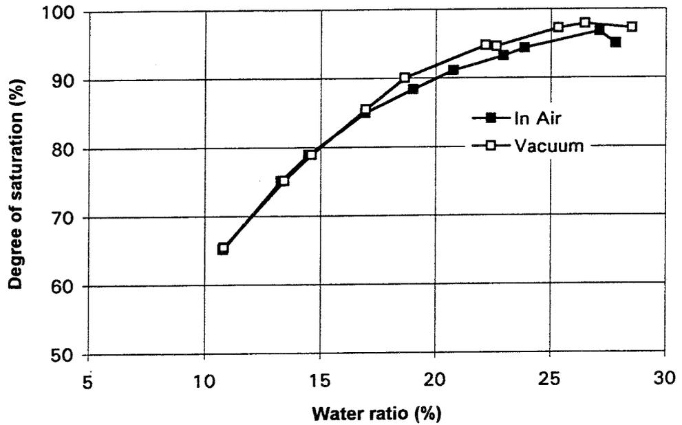
*Figure 4-17. Degree of saturation as a function of water ratio for samples compacted in air and during vacuum.*
