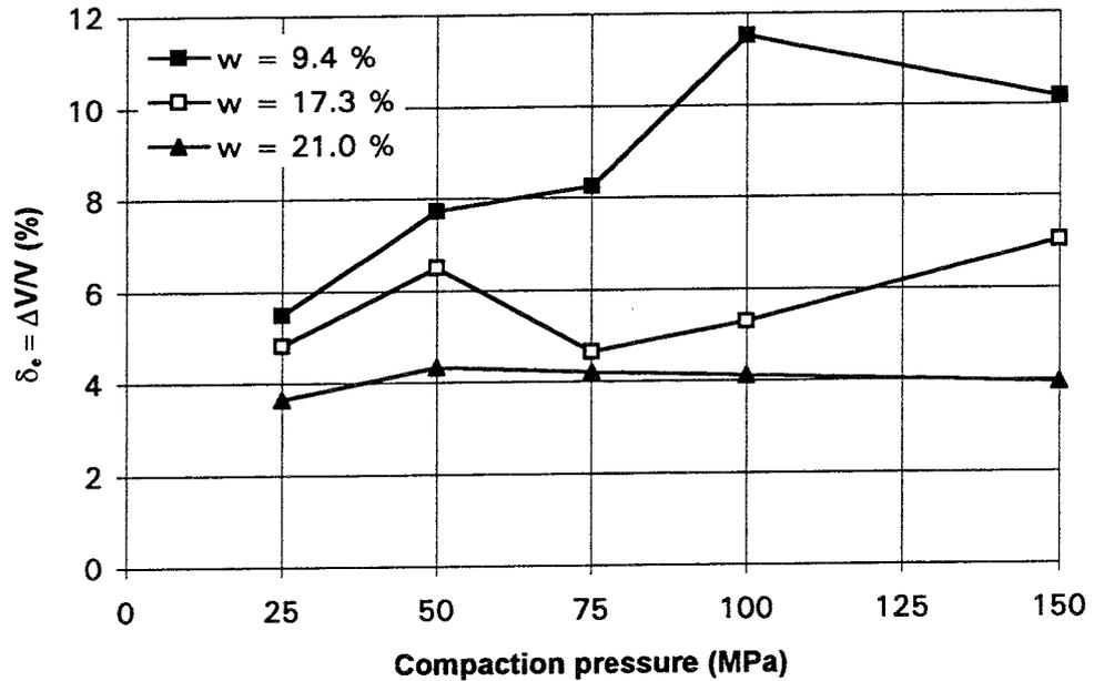
*Figure 4-13. The expansion ratio as a function of the compaction pressure for MX-80 samples compacted at different water ratios..*
