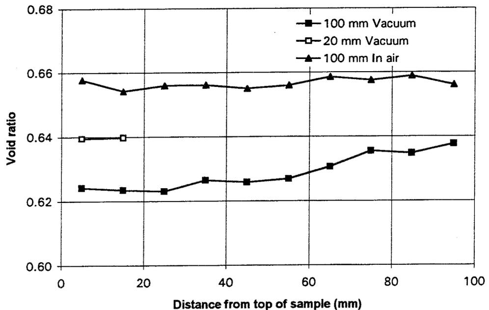
Figure 4-19. The void ratio plotted as a function of the distance from the top of the sample. Water ratio  $\approx 21\%$ .
