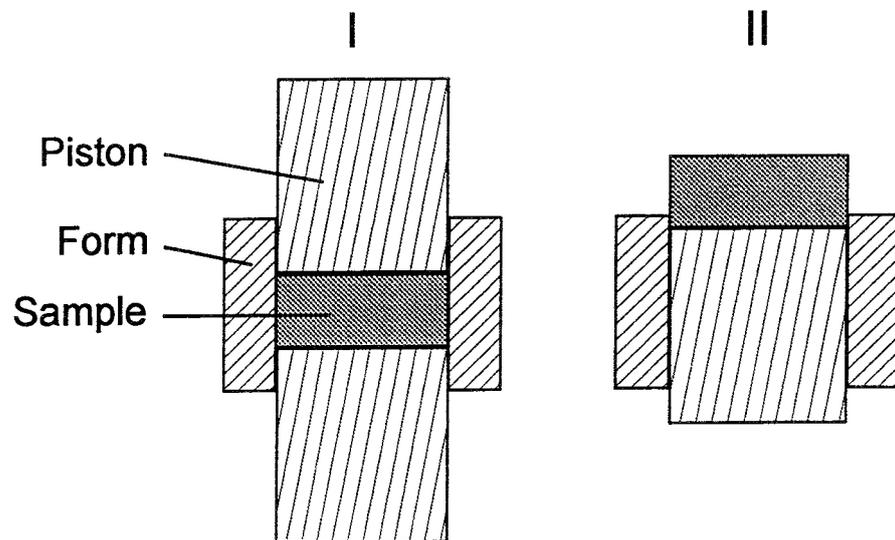
*Figure 5-1. Schematic drawing of the technique used for pushing a block out of a form.*
