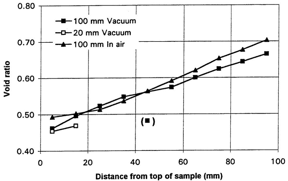
Figure 4-18. The void ratio plotted as a function of the distance from the top of the sample. Water ratio  $\approx 9\%$ .
