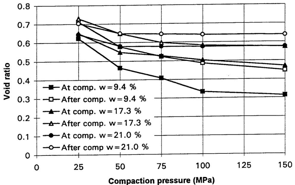
Figure 4-11. The void ratio as a function of the compaction pressure for samples with different water ratio.
