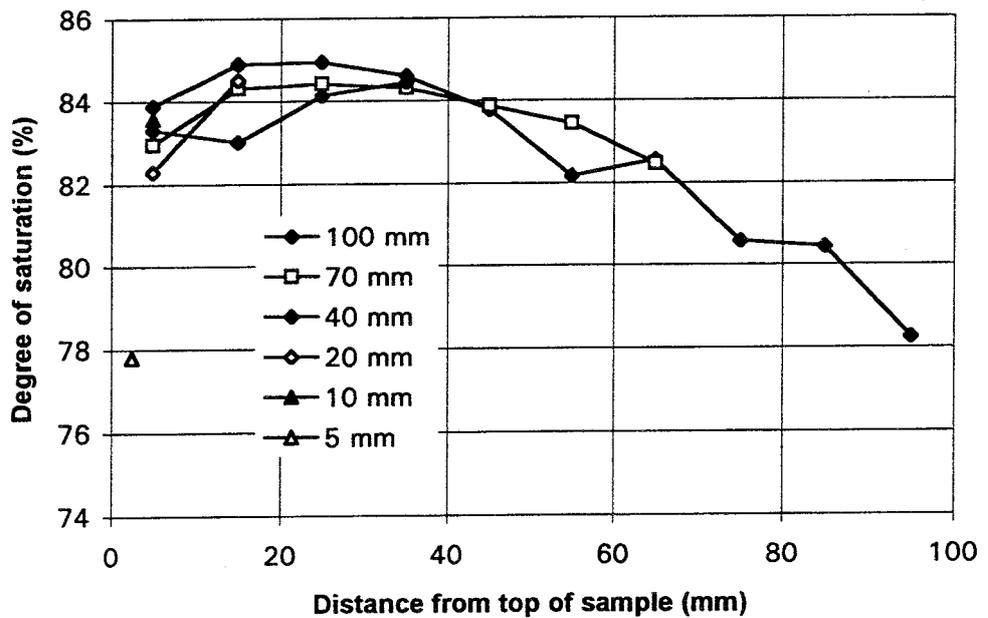
*Figure 4-6. Void ratio (a) and degree of saturation (b), plotted as functions of the distance from the top surface of the sample for different sample heights. Water ratio = 18%.*
