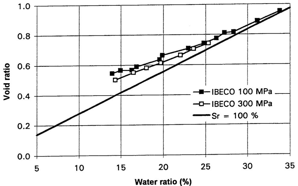
*Figure 4-8. The void ratio as a function of water ratio for MX-80 (a) and IBECO-Na (b). Compaction pressure = 100 MPa and 300 MPa*
