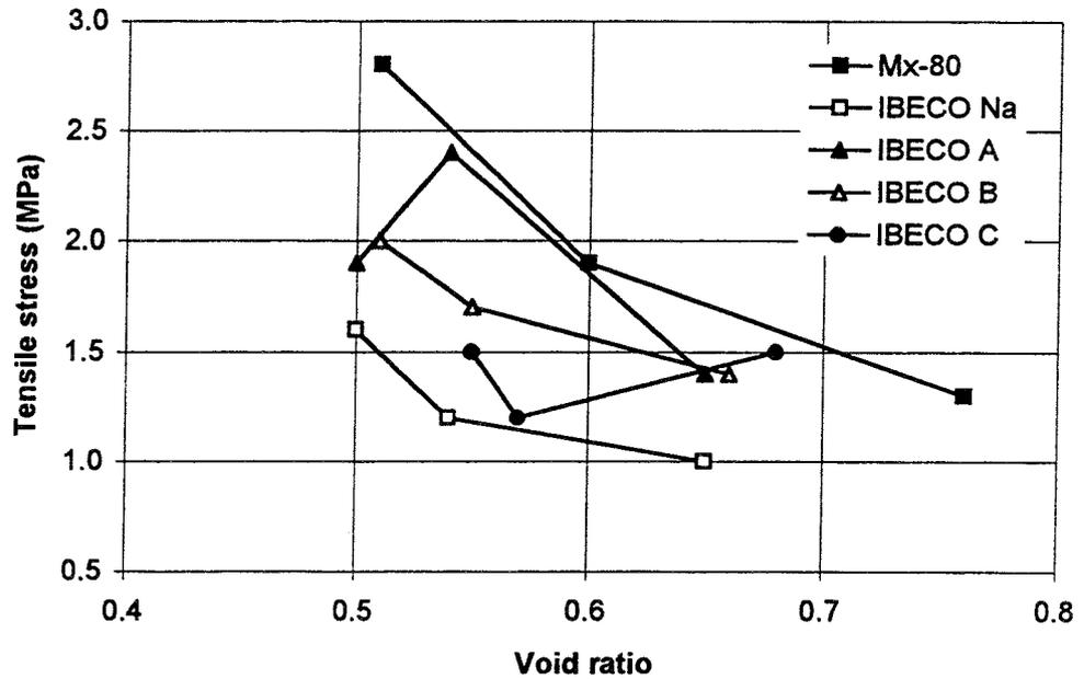
Figure 6-5. Tensile stress at failure as a function of void ratio for different bentonites.
