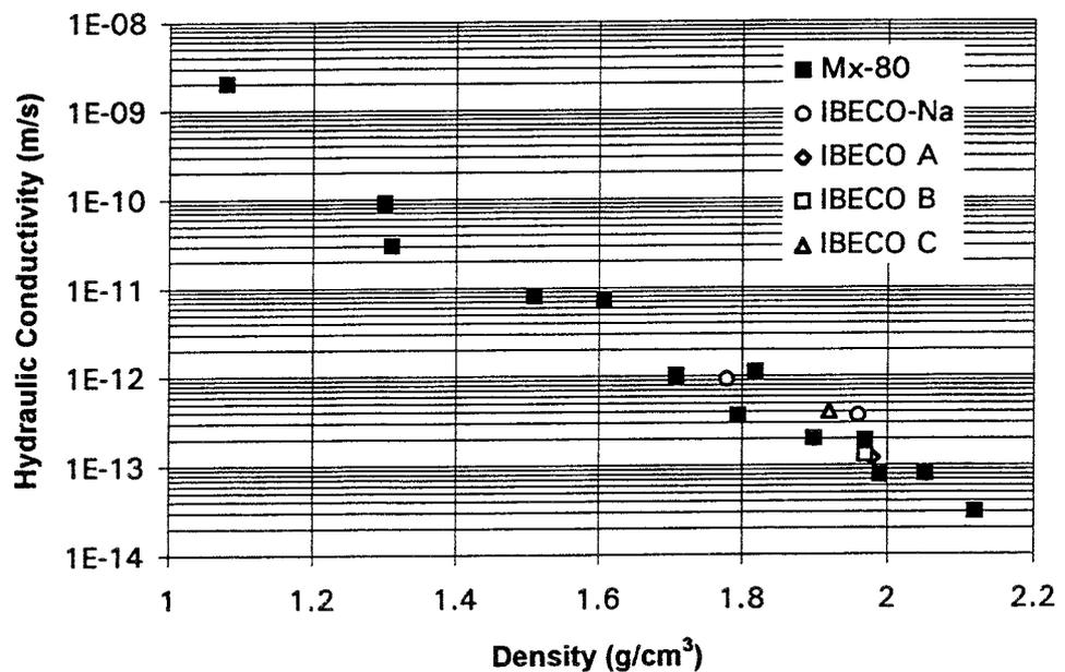
**Figure 6-7.** Hydraulic conductivity of the bentonites as a function of the density at saturation.
