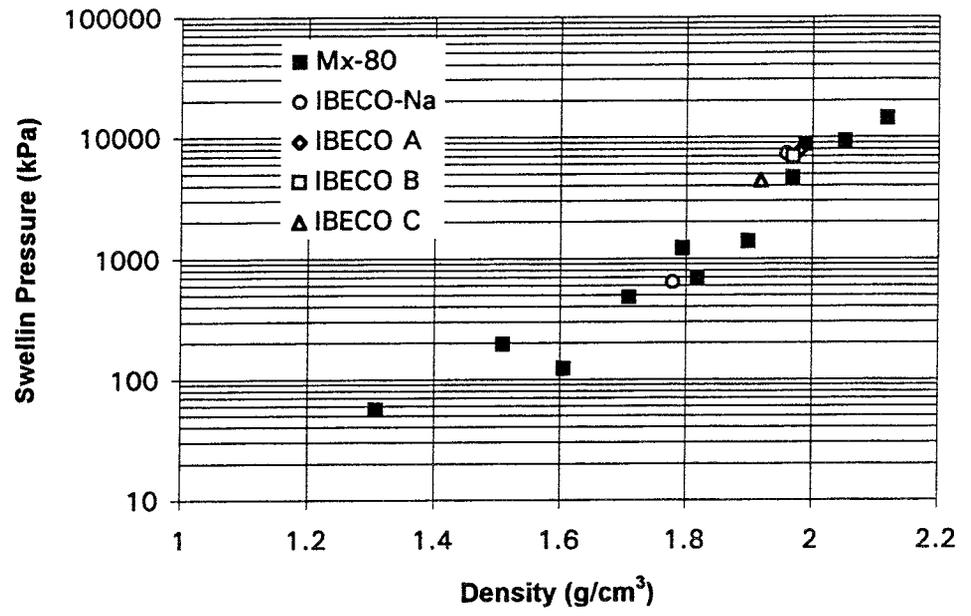
*Figure 6-8. Swelling pressure of the bentonites as a function of the density at saturation.*
